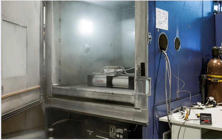
A2A Booster undergoing Low Temperature cycle testing
