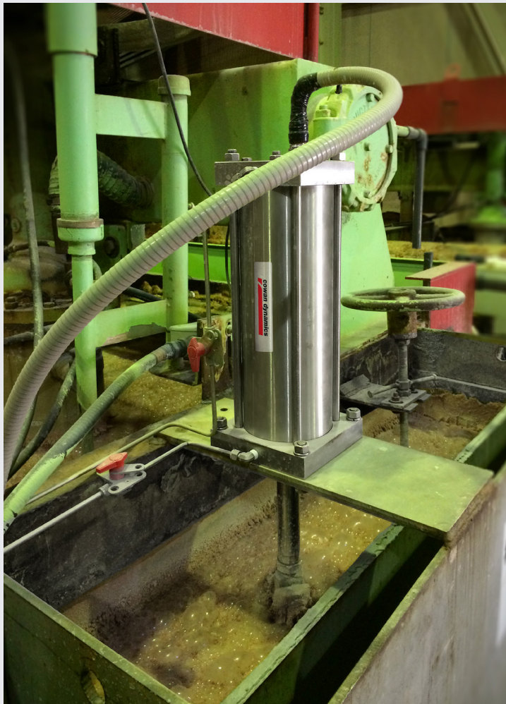
8" Bore Stainless Steel AT Series with remote positioner in a potash plant
