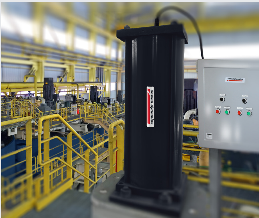
14" Bore AT Series with pneumatic control panel, operating a dart valve in a mining flotation cell application
